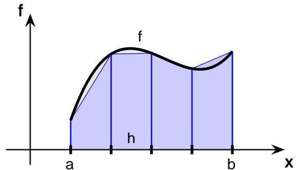
$$I_a^b(f) = \sum_{i=0}^{N-1} I_{x_i}^{x_{i+1}}(f), \quad \text{Trapezregel: } I_{x_i}^{x_{i+1}}(f) \approx \frac{h_i}{2}(f(x_i) + f(x_{i+1}))$$
