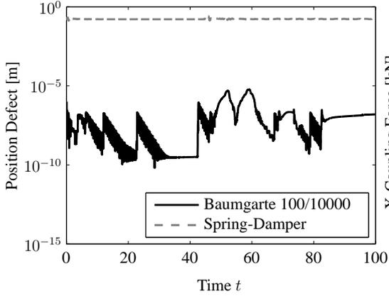
Fig. 10. Position defect between vehicle and trailer.
