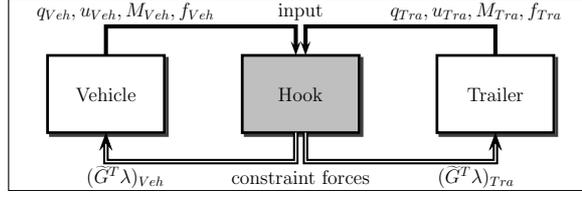
Fig. 9. Model structure for vehicle-trailer coupling in veDYNA.
