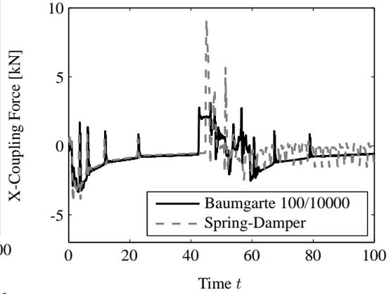
Fig. 11. Coupling forces between vehicle and trailer.
