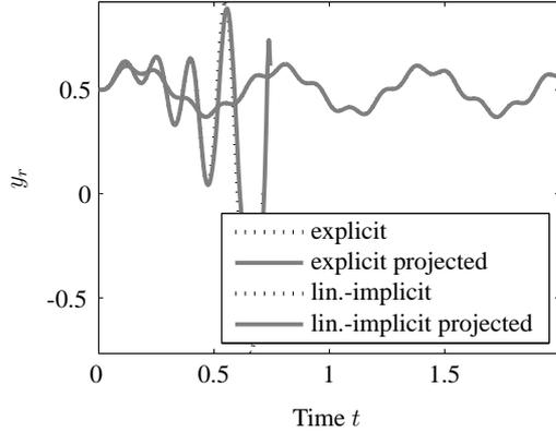
Fig. 7. Benchmark “Car axle”: Explicit and (partitioned) linear-implicit Euler method.
